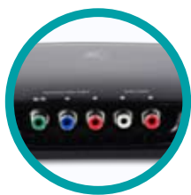
The YPbPr and audio connectors flanking the left panel of the M200. At the rear panel are the HDMI, coaxial, and LAN ports.
